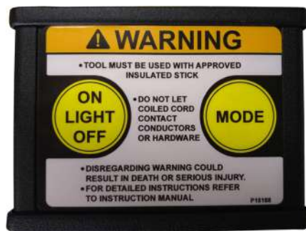
TOP DISPLAY OF VOLT METERS
